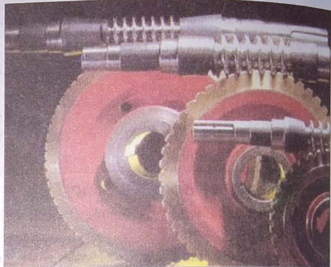
Hardened and ground worm shaft and worm wheel pair
