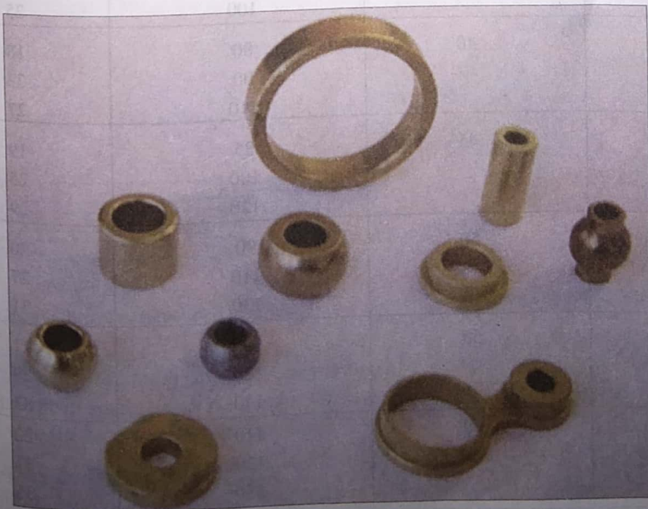
Oilless bearings made using powder metallurgy.
