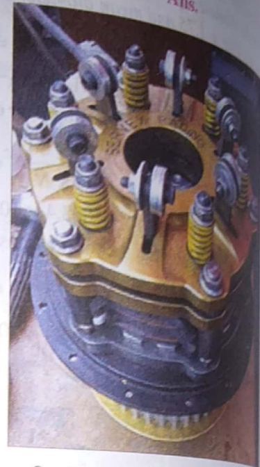
Centrifugal clutch with three discs and four steel float plates.
